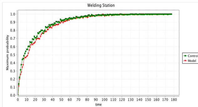
Figure 5: Maximum Fault Occurrence Probability for the Welding Station PBN vs Control
